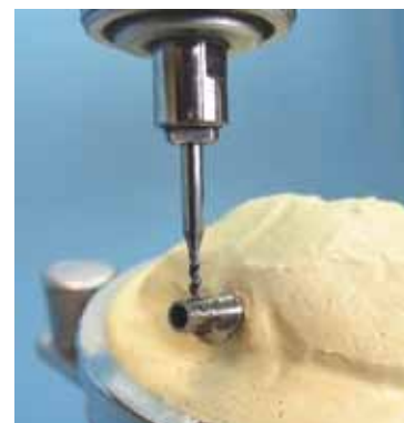
Drilling the hole before cutting the thread.
