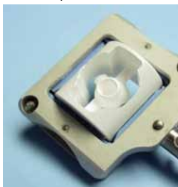
Milled crown made from "Cercon". (Degudent).
