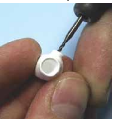
Use a 30% larger primary drill to allow for shrinkage.
