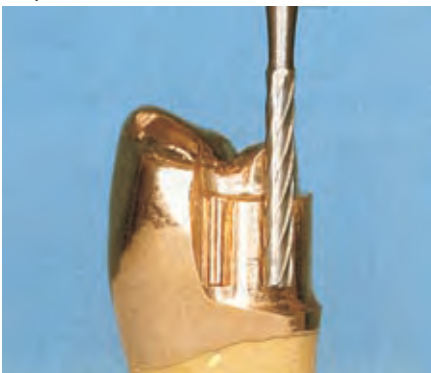
Remilling of the groove is carried out with the tool, F5382H10. During this process the groove bur should only be moved vertically in the slot.
