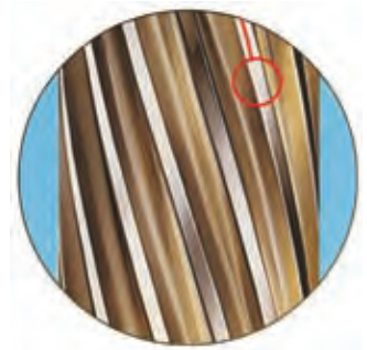
Close up view of the helical tooth used for smooth milled surfaces and chip removal.
